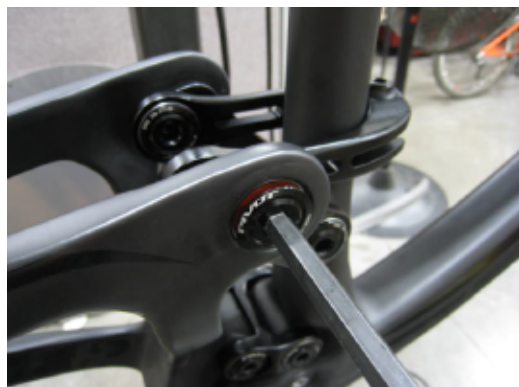
49 Install upper bolts in RT
