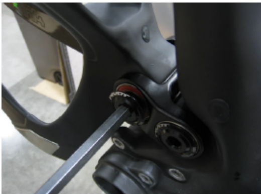
46 Install RT Bolts
