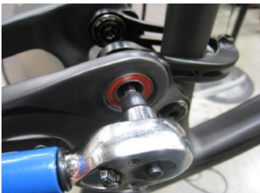
48 Clevis bolts may be torqued to 35Nm at this time if not done previously
